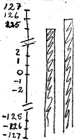
The quantizing steps in PCM are not linear in order to enhance the signal to distortion ratio. For example, a coding scheme called A-law is used. By using a greater number of quantizing steps for signals of low amplitude and smaller number of quantizing steps for signals of large amplitude, a reduction in the overall signal distortion is achieved.
