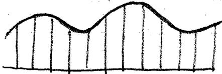
The result is a pulse amplitude modulated (PAM) signal (see figure below)
