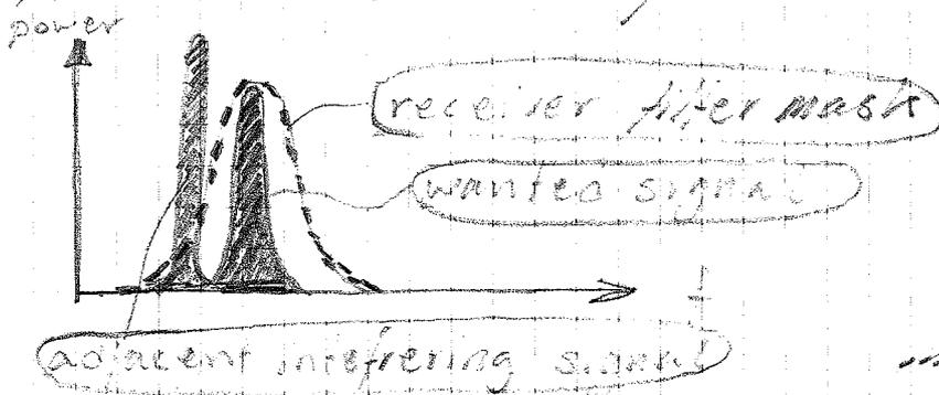
Some of the energy from the (adjacent signal in frequency) will slip through the receiver filter mask and become an interfering signal.
