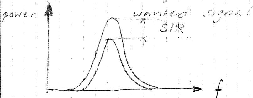
B. Adjacent channel interference, is interference from signals which are adjacent in frequency to the desired signal. Adjacent channel interference results from imperfect receiver filters which allow nearby frequencies to leak into the pass band of operation.
