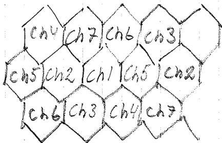
A way to further increase the space division is to divide the cells into sectors with directional antennas
