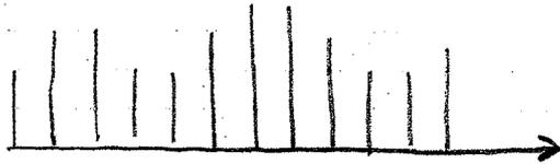
In order to digitize the signal the height of each pulse must be quantized.
