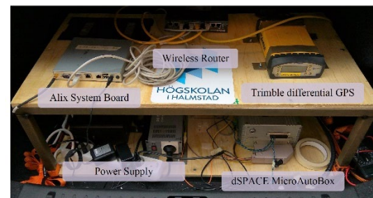
Figure 5.2: The trunk of the competition car with its devices.
